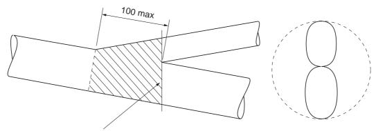
The largest minimum combined **boom spar cross section** over the length of the junction is found in this section and it shall not exceed 40 mm.
